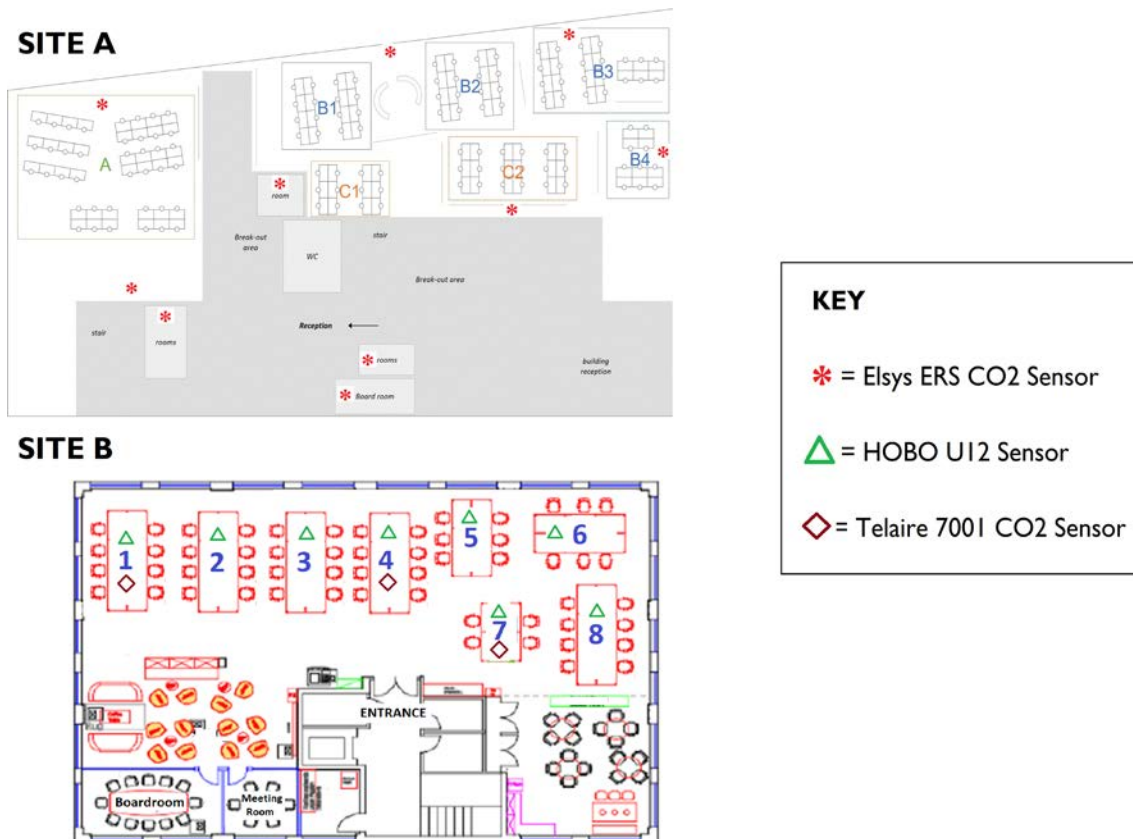
Figure 2: The floorplans, including sensor locations, for the two sites in the follow-up study
